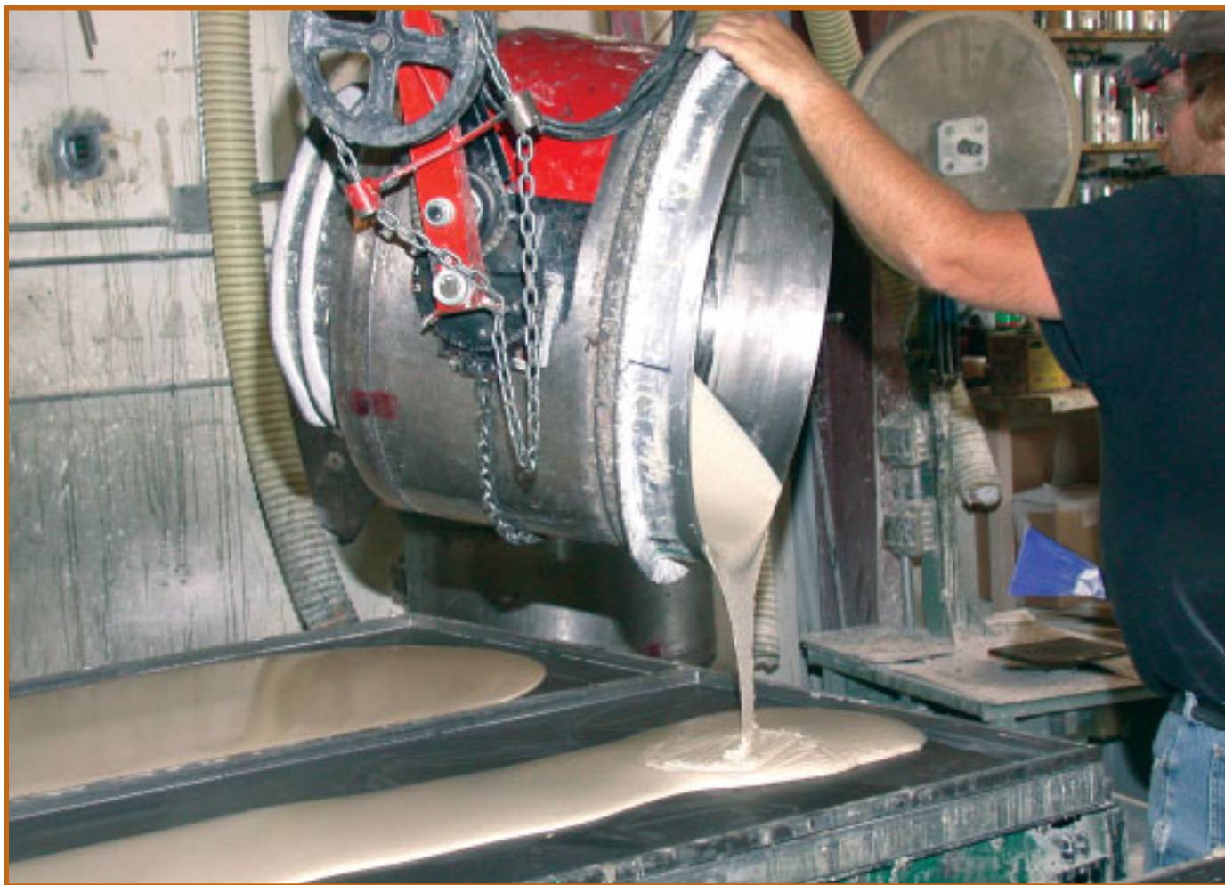
Solid surface sheets are cast on stainless steel molds and sanded to 1/4 in. after curing.
