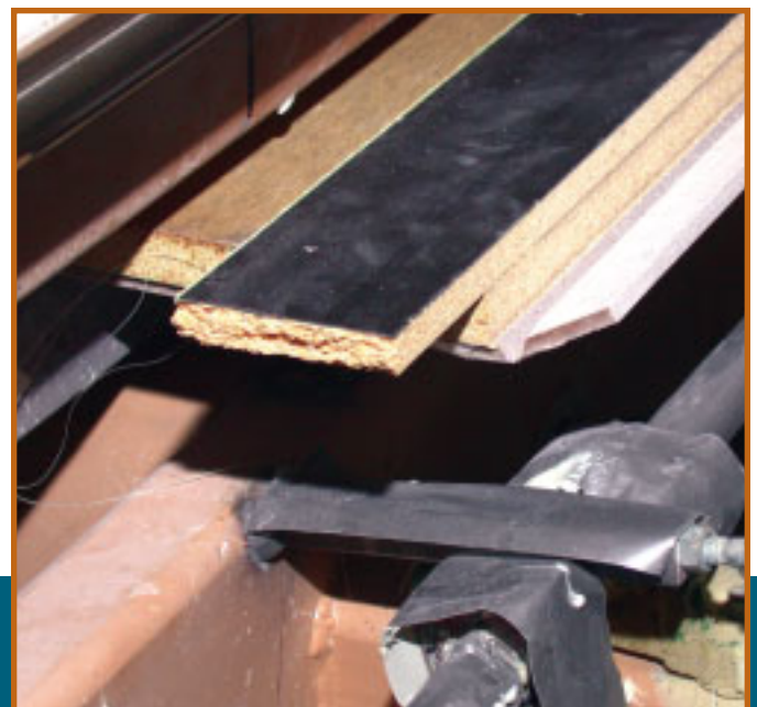
Once the joint has been filled with adhesive, the v-grooved edge is automatically folded together in the machine.
